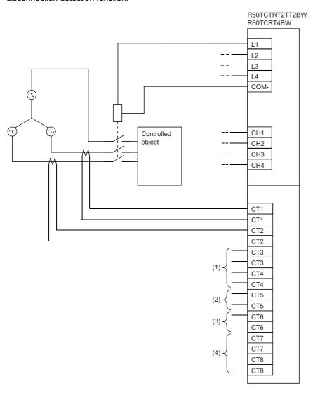
The disconnection of the three-phase heater is detected by measuring the currents of two of the three cables. In the above wiring example, set "CT input channel assignment setting" of "CT setting" as indicated below.
